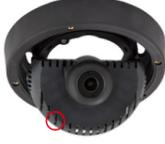
The LED now flashes once and repeats the flash signal after pausing for one second (the number of flashes indicates the current boot option). To go to the next boot option, briefly press the key again (< 1 sec). After the last boot option, the camera returns to the first option (LED flashes once).
