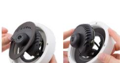
Now take the disc and pull it gently apart at the cut. Place the disc around the cables where the sealing and the housing meet. Push the disc down on the opening in the housing.
