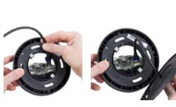
board support to get to these screws. Insert the screws with washers and tighten them.
