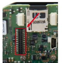
Use one finger to carefully press the board of the module onto the receptacle. Make sure that the MxIOBoard-IC is fully inserted.
