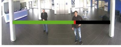
Carefully turn the lens using the red lens wrench in clockwise or counter-clockwise direction until the red area of the focusing aid in the camera image is as small as possible.
